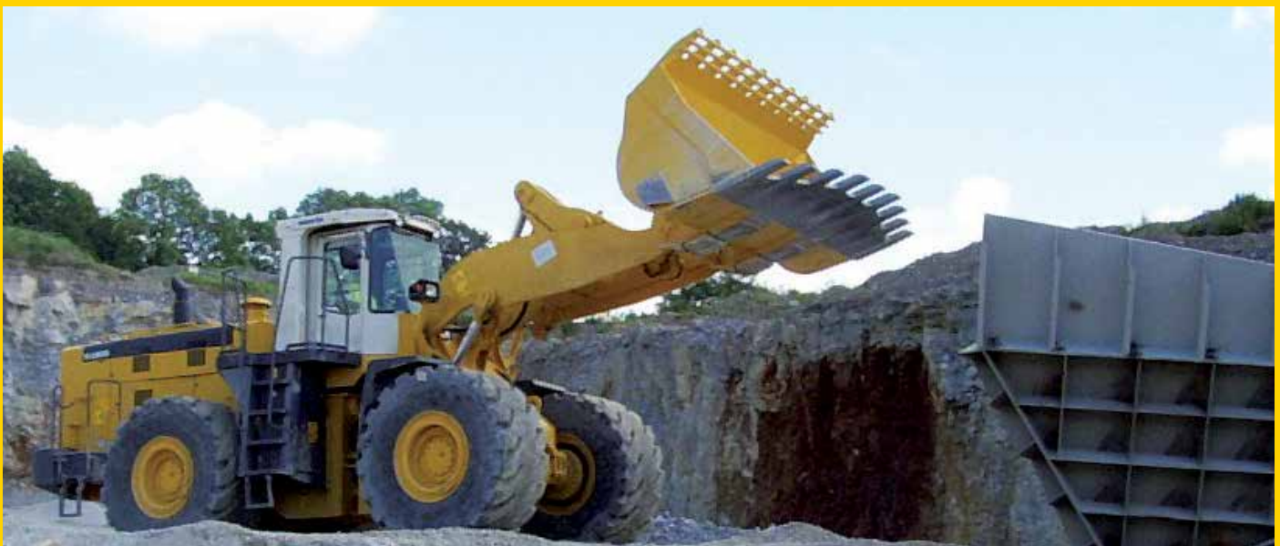
Spade shaped serrated bucket lip
